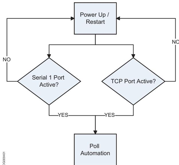
Flow Diagram for **Automation Automatic IP Fallback Mode (3)**
