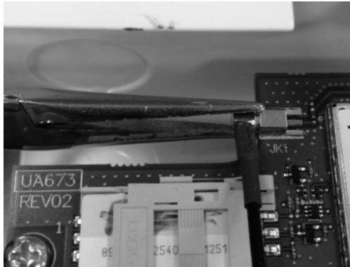
3. Carefully disconnect the cellular antenna from the cellular radio module on the 3G4010. To remove the cable from the radio module, use needle nose pliers, grip the antenna connector and pull out, directly away from the PCB antenna socket. (see photo above.)
