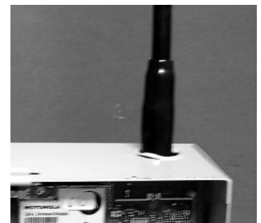
Extension antenna connected
