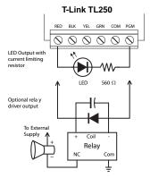
**PGM2**-The PGM2 output is dedicated as an input follower that is triggered on any input alarm (including Bell Follower which generates Burglary and Fire Alarms) except for keyswitch zones. The PGM2 output will only turn off when ALL violated zones are restored.
