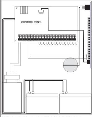
INSTALL BATTERY AND AC WIRING AS SHOWN ABOVE IMPORTANT: A minimum ¼" (7mm) separation must be maintained at all points between battery/primary AC wiring and all other wiring and connections.
