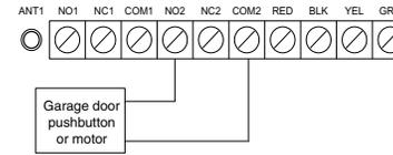
Connect an output of the PC5102-433 across the wall-mounted push button or directly at the motor of the garage door opener (please consult the garage door opener instructions for proper connections). Set up the system and wireless key so that it is programmed to pulse an output for a short duration (5 seconds) so that every time the programmed key is pressed the garage door is opened or closed. The system can also be set up so that
