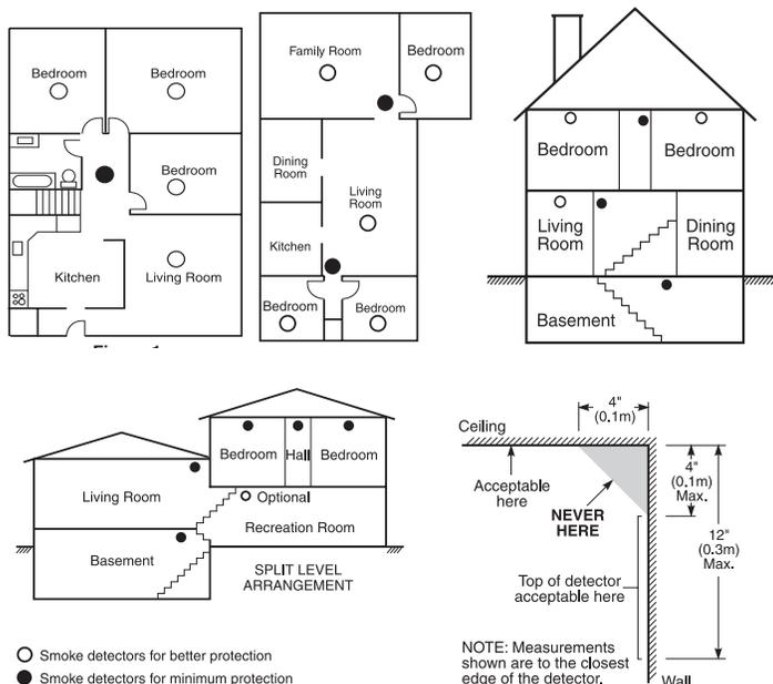
\*\* *Smoke detectors should always be installed in accordance with CAN/ULC-S553-02 standard for installation of smoke alarms.*
