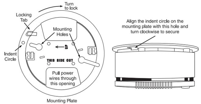
The Meridian smoke alarm mounts to a standard 4" octagonal electrical box. **12 to 24VDC or Full Wave Rectified power must be supplied from a ULC Listed power supply or the auxiliary power terminals of a ULC Listed alarm control unit. Wiring should be in accordance with the Canadian Electrical Code, Part I, and applicable local codes.**
