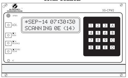
**Liquid Crystal Display:** 2-line, 16 character per line liquid crystal display; backlit for easy reading in low level light
