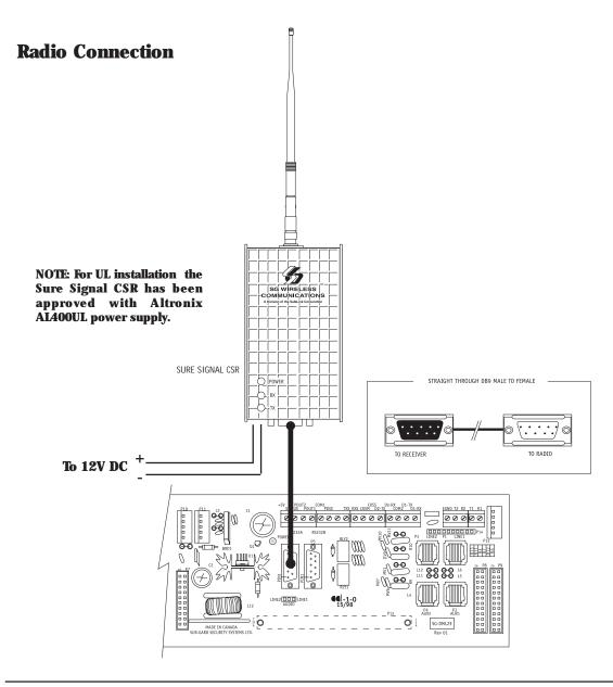
The serial connection is a straight through 9 pin male to 9 pin female connection.
