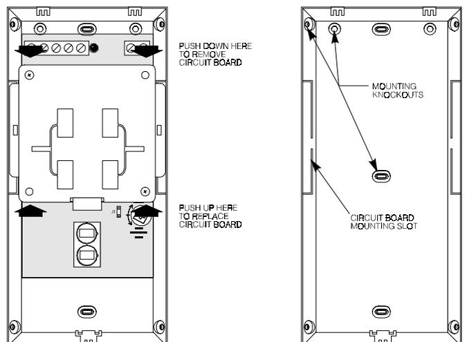
With the circuit board removed, use a small screwdriver to punch out the wiring and mounting knockouts located in the detector's back. Feed the wiring through the wiring knockout and secure the detector to the wall.
