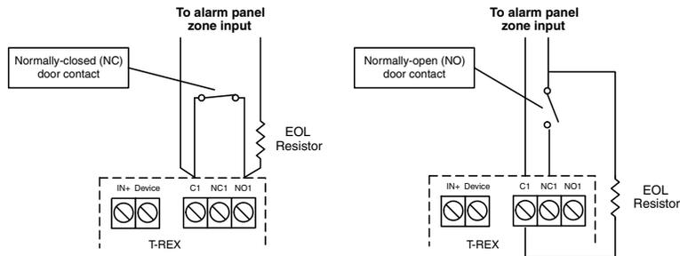
**NOTE:** The EOL resistor should be located within the T.Rex housing to provide proper supervision.
