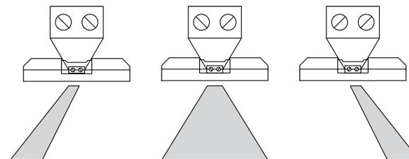
2. Rotate the barrel assembly up or down as required. This will adjust the detection zone away from or towards the door respectively. If the detector is mounted directly above the door, it is recommended that the detection area be directed away from the door. To achieve this, rotate the barrel assembly so that the lower edge of the detector lens is about 1/4" above the edge of the case.
