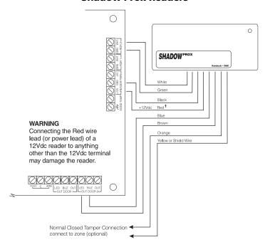
\*NOTE: Only use the +12V power supply when using the Shadow Prox Reader.
