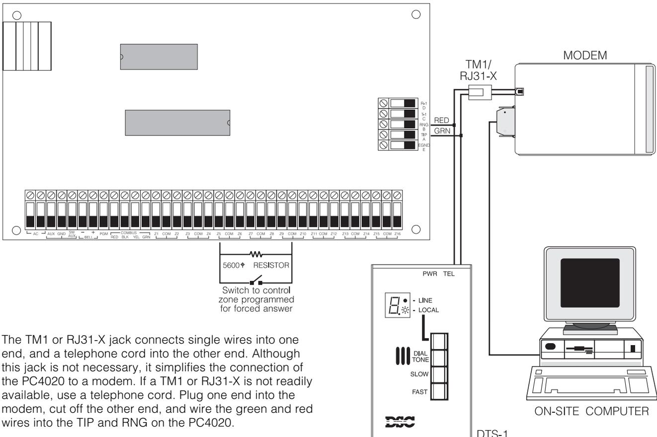
The TM1 or RJ31-X jack connects single wires into one end, and a telephone cord into the other end. Although this jack is not necessary, it simplifies the connection of the PC4020 to a modem. If a TM1 or RJ31-X is not readily available, use a telephone cord. Plug one end into the modem, cut off the other end, and wire the green and red wires into the TIP and RNG on the PC4020.
