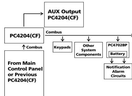
**NOTE 5:** If the PC4204CF is not set up for Combust repower, include the current drawn by the downstream components in the standby battery calculation for either the previous PC4204CF or the main panel.
