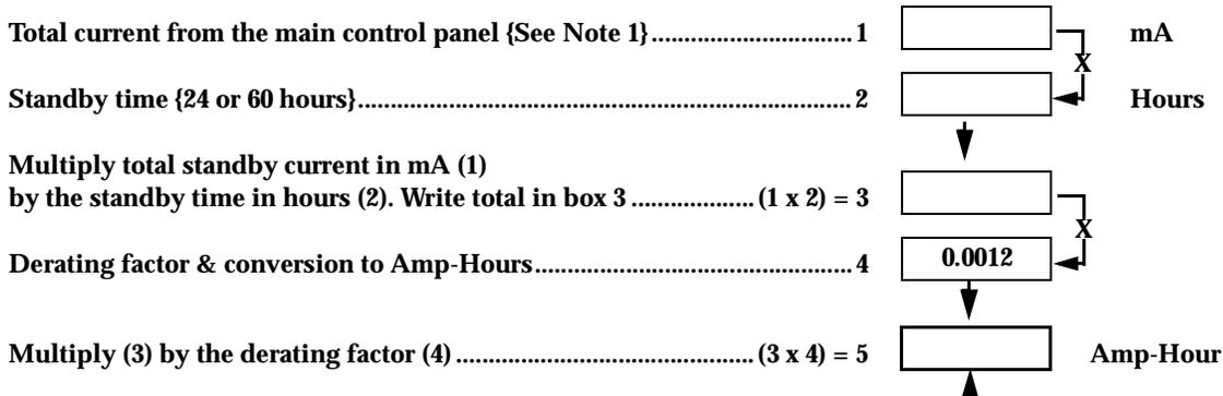
**This is the minimum size battery required to maintain the main panel for the standby time selected**
