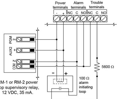
The type of smoke detector must be latching. To reset the smoke detector, refer to the panel installation manual.
