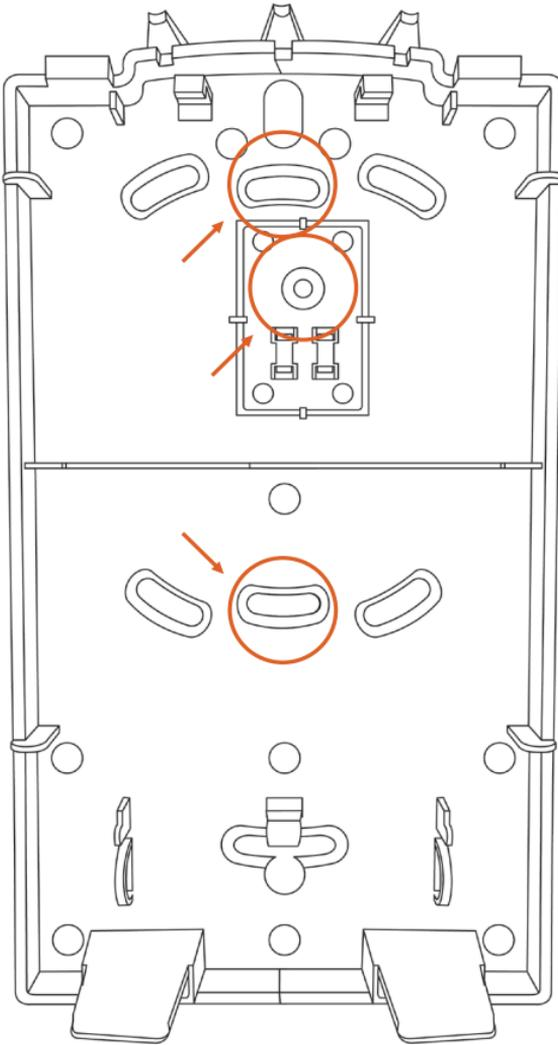
Set the back plate aside and drill holes at the mounting locations.
