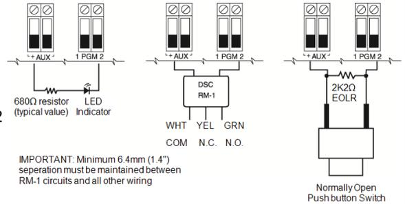
IMPORTANT: Minimum 6.4mm (1/4") separation must be maintained between RM-1 circuits and all other wiring
