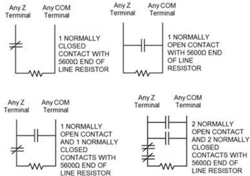
**Double End-of-Line Resistor wiring**
