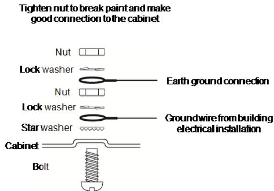
**Figure 2-18 Ground Installation**
