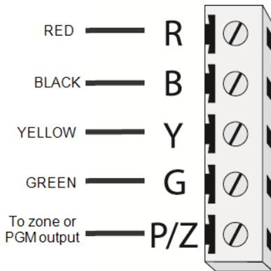
**Figure 2-8 Keypad P/Z Terminals**
