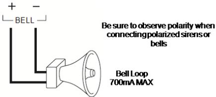
**Figure 2-13 Bell Wiring**
