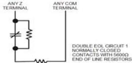
**Figure 2-11 DEOL Wiring**
