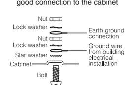
**NOTE:** Using an insulated green wire (minimum 22AWG), connect the GEND terminal on the Corbus and the grounding wire from the building electrical installation to any of the available holes on the back or side of the metal cabinet. See the diagram attached to the cabinet for suggested GND point location and hardware recommendations.
