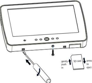
4. Secure keypad backplate to wall using mounting holes. (See Figure 2.) Use all 4 screws provided unless mounting on a single gang box. Use the plastic anchors supplied if the unit is to be mounted on drywall. If using the keypad tamper, secure the tamper plate to the wall with a screw.
