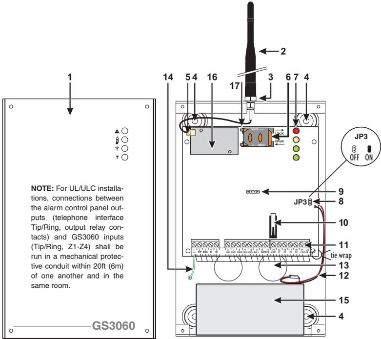
All circuits are classified for UL installations as Power Limited/Class II Power Limited except for the battery leads which are not power limited. Do not route any wiring over circuit boards. Maintain at least 1" (25.4mm) separation. A minimum 1/4" (6.4mm) of separation must be maintained at all points between Power Limited wiring and all other non-Power Limited wiring. Route wires as indicated above.
