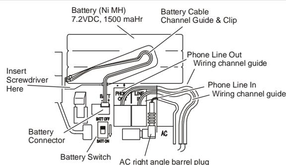
**NOTE:** Battery life is 4-5 years under typical operating conditions. Replace Battery every 4-5 years. Battery capacity deteriorates with age and number of charge/discharge cycles.
