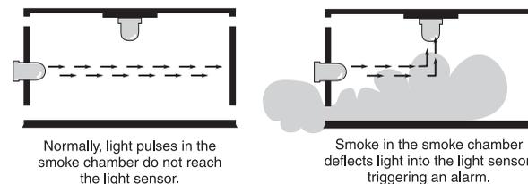
As shown in the illustration, a light source is directed across the smoke chamber and is not normally reflected into the sensing element. When smoke enters the chamber, the light beam is scattered by the smoke and reflected into the sensor. When enough light is detected by the sensor, an alarm is activated. On alarm, the sounder is activated and the red LED will flash. **When the smoke clears from the smoke chamber, the unit will automatically reset itself.**
