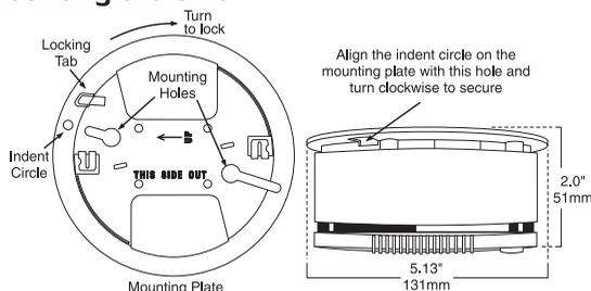
Locate the smoke detector mounting plate on the wall or ceiling and mark all desired screw locations\*. Use the supplied wall anchors for all screw locations. When the anchors have been placed, secure the mounting plate to the ceiling or wall.
