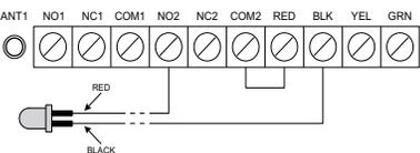
The LED can be used to indicate whether the system is armed or disarmed. If the output is programmed as an armed status output, the red LED will turn on when the system is armed and will turn off when the system is disarmed.
