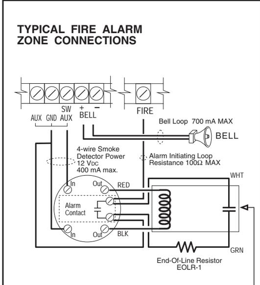
Note: Smoke detector must be 4-wire ULC listed latching type (ESL 446C). To reset smoke detectors - press [\*] then hold down key [4] for 2-3 sec.
