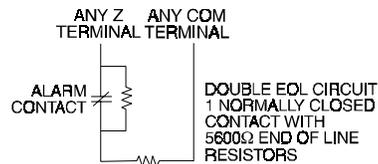
**!** *This option can only be selected if Normally Closed (NC) detection devices or contacts are being used (ie: Do not use DEOL resistors for Fire zones or LINKS Supervisory zones). Only one NC contact can be connected to each zone. Multiple detection devices or contacts on a single loop is not allowed.*
