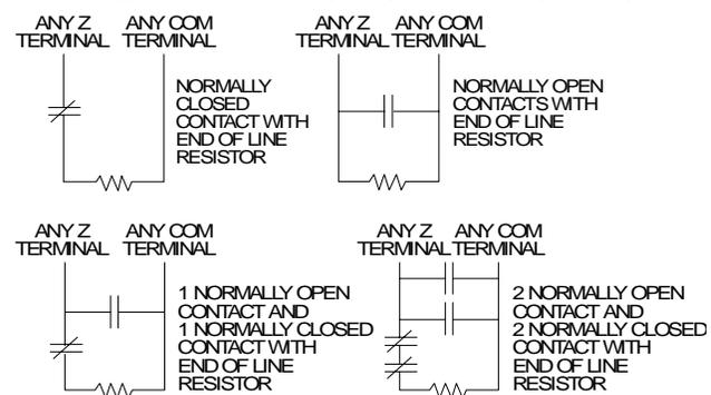
**!** *This option should be selected if either Normally Closed (NC) or Normally Open (NO) detection devices or contacts are being used.*
