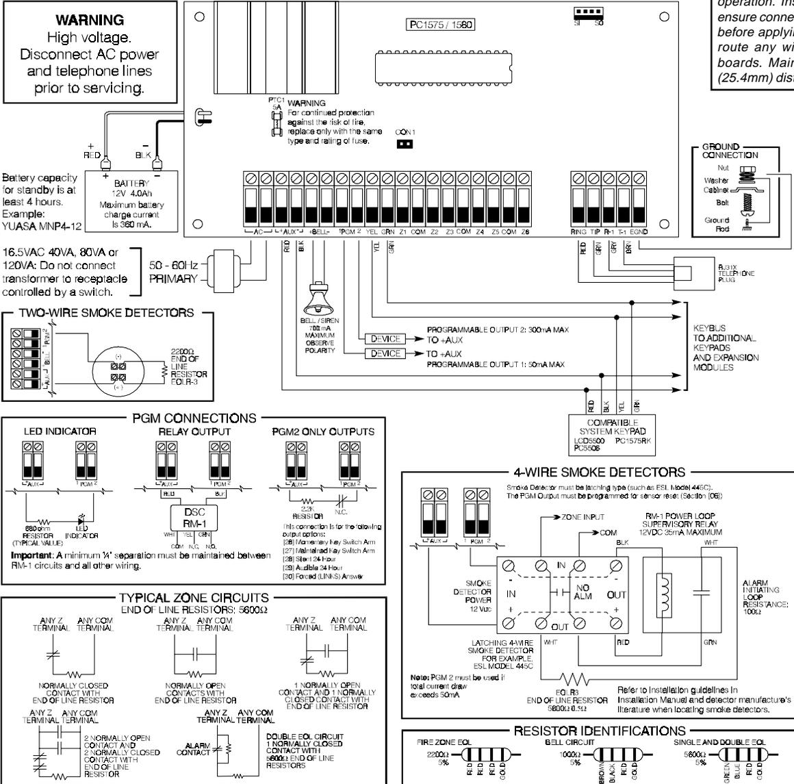
Incorrect connections may result in fuse failure or improper operation. Inspect wiring and ensure connections are correct before applying power. Do not route any wiring over circuit boards. Maintain at least 1" (25.4mm) distance.
