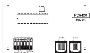
The PC5400 Printer Module will allow the panel to print out all events that occur on the system to any serial printer. The printout will contain the time, date and the event that occurred (see Section – 5.25 “On-site Printer”).
