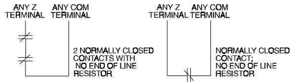
**!** *This option should only be selected if Normally Closed (NC) detection devices or contacts are being used.*
