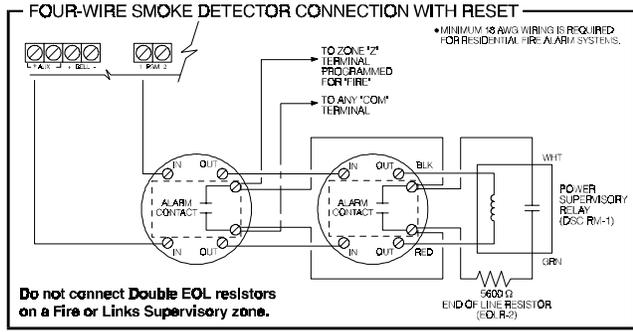
Do not connect Double EOL resistors on a Fire or Links Supervisory zone.
