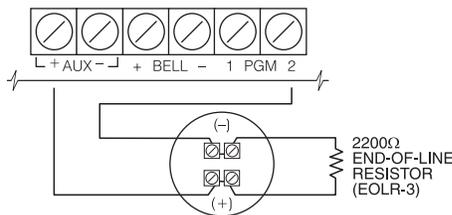
**!** If PGM2 is programmed for 2-wire smoke support, the connector JP1 on the main board must be removed.
