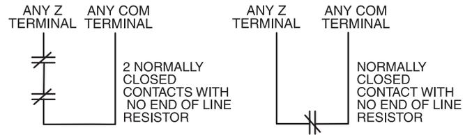
To enable normally closed loops, programming section [013], option [1] must be ON.
