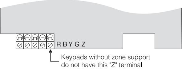
"Z" version keypads are also indicated by a label located on the back of the keypad plastic. The label reads: "Z" version.
