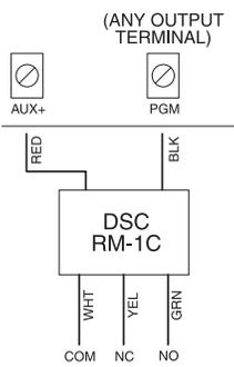
PGM1 can sink up to 50mA of current. Connect the positive side of the LED or buzzer to AUX+, the negative side to PGM1. If more than 50 mA of current are required, a relay must be used. Please study PGM wiring in the accompanying diagram.
