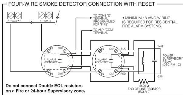
Do not connect Double EOL resistors on a Fire or 24-hour Supervisory zone.
