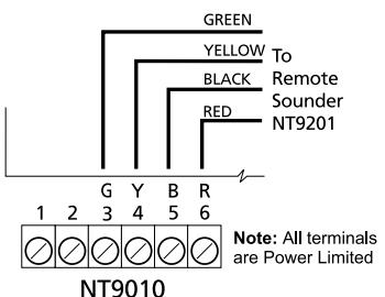
For the sounder to work on the system you must turn on the **Remote Annunciation** option (section [017], option 5). When this option is turned on, the remote sounder will also be supervised. If the NT9201 does not report a supervisory signal within 30 seconds, a "Remote Bell Trouble" will be generated and logged in the event buffer.
