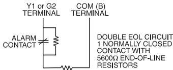
In this configuration the system should see 5600 Ω in the normal state. If the zone becomes open, the system interprets this as a tamper. If the zone becomes short circuited the system will interpret this as a fault. If the system sees 11,200 Ω the system will interpret this as a zone violation and will go into alarm. To program the system for this configuration, set section [013] option [1] to OFF and option [2] to ON (see Chapter 5: Advanced Programming).
