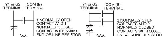
In this configuration the system should always see 5600Ω when the zone is not violated. If the zone becomes open or short the system will go into alarm. There is no supervision or tamper detection of zones. To program the system for this configuration, enter Advanced Programming (see section 5) and set section [013] option. [1] to OFF and option [2] to OFF.
