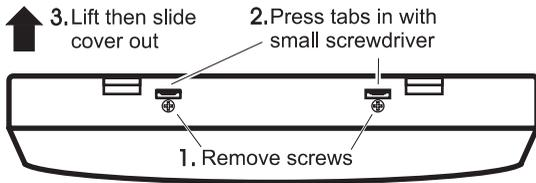
1. Place the unit face down on a surface that will not scratch or mar the front cover.
