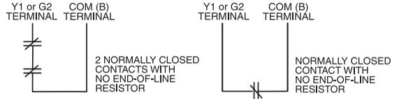
In this configuration there is no supervision or tamper detection of zones. An open condition will sound an alarm; a short circuit condition will not be indicated. To program the system for this configuration, enter Advanced Programming (See Chapter 3) and set section [013] option [1] to ON.
