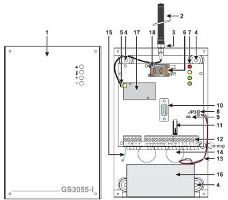
All circuits are classified for UL installations as Power Limited/Class II Power Limited except for the battery leads which are not power limited. Do not route any wiring over circuit boards. Maintain at least 1\* (25 4mm) separation. A minimum 1/4" (6.4mm) separation must be maintained at all points between Power Limited wiring and all other Non-Power Limited wiring. Route wires as indicated in the diagram.
