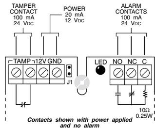
**NOTE:** This unit is UL Listed and should be connected to a listed control unit or power supply providing at least 4 hours of standby by power.
