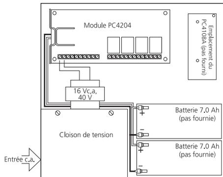
INSTALLEZ LE CÂBLAGE BATTERIE ET C.A. CONFORMÉMENT AU DIAGRAMME CI-DESSUS
