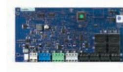
**Power Supply with Corbus Repeater (HSM3204CX)**
