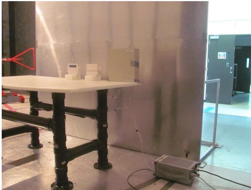
Photo 8.1-1: Conducted emissions setup
