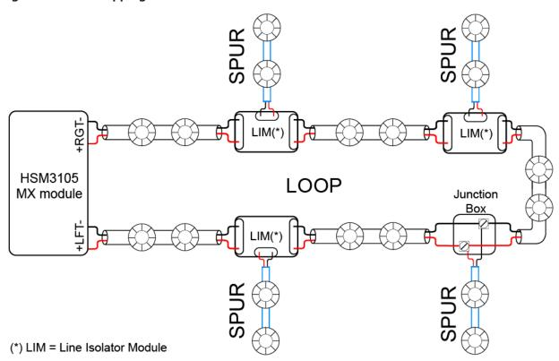
If multiple spurs are required for the installation, then you can use multiple MX920 Isolator modules. These spurs can be applied to either two wire or four wire MX loop configurations. Refer to the MX920 manual for more details on the isolator modules. See Figure 7.
