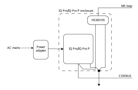
Figure 2: Low Power Mode - External Mount
