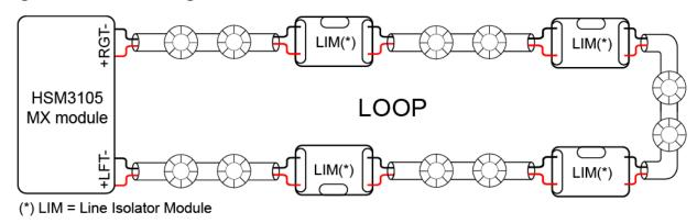
You can configure a HSM3105 module using a loop configuration or four wire wiring. See Figure 6. In the case of a single wiring trouble, for example a cable break or short circuit trouble, all the devices can still be managed, depending on the isolators that are present on the loop.
