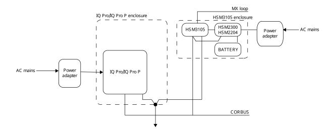
Figure 4: High Power Mode - wiring diagram
