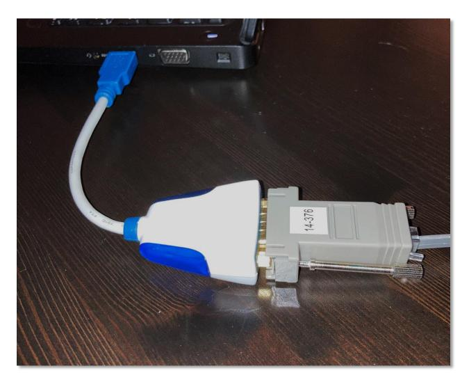
**9.** Connect the other end of the PC-LINK cable to the PC. If the PC has a DB9 COM port available you can connect the PC-Link DB9 connector directly to it. Otherwise, plug the PC-LINK DB9 into the USB to Serial DB9 connector, and then plug the USB end into a USB port on your PC.
