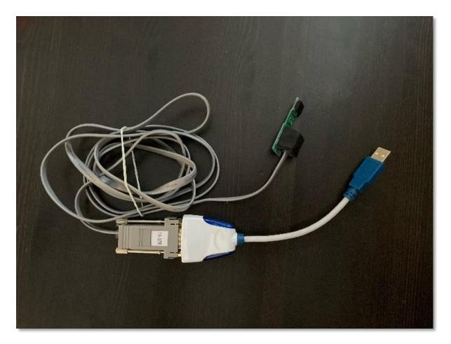
**7.** Pictured above is the kit called "PC-LINK-USB". This kit includes the PC-LINK header, cable, DB9 connector and USB to serial adapter. The USB to Serial adapter included in the PC-LINK kit is currently the only adapter recommended for use with the DLS 5 software.
