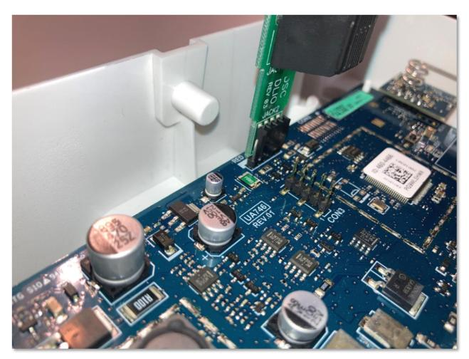
**8.** Notice the orientation of the 4 pin PC-LINK header on the PGXWLSHW8 PC-LINK five pin connector. The header must be connected on pins 2 to 4 (from left to right) and inverted to the typical orientation for other DSC/JCI products. Pin 1 should be sticking out alongside the PC-LINK header as in the photo.
