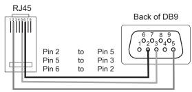
• SG-DRL3 Debug Output: Connect the RJ-45 end of the debug cable to the debug output jack on the front of the line card. Connect the female DB-9 connector to the serial port of a computer (COM1 port - DB-9 male).
