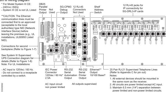
WARNING: To reduce the risk of electric shock the product is provided with a grounding type power supply IEC receptacle. Connect product using an appropriate IEC cable to a grounded receptacle.
