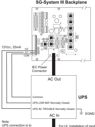
For UL/ULC installations use a UL listed UPS (Uninterruptible Power Supply) for protective-signaling systems and/or listed burglary alarm power supply, as applicable.
