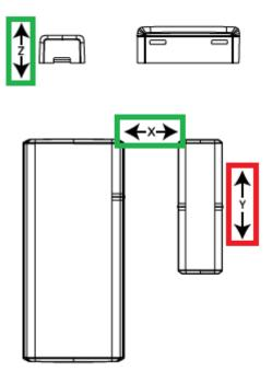
To minimize the potential occurrence of the issue, the PGx303 PowerG Wireless Magnetic Door/Window Contact must be installed vertically on a door that slides open horizontally, or horizontally on a window that slides open vertically.
