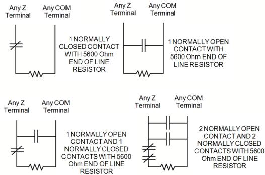
**Double End-of-Line Resistor wiring**
