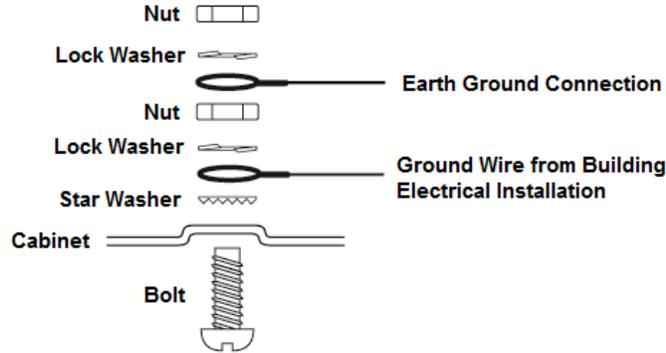
**Figure 2-18 Ground Installation**
