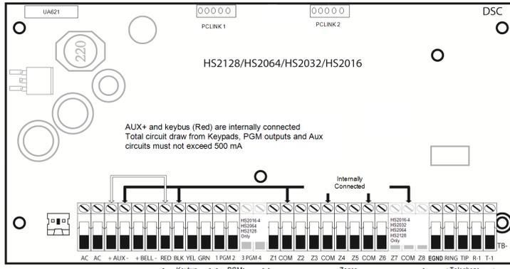
**Figure 2-2 Wiring Routing (EN50131 only)**
