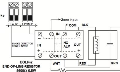
Smoke detector must be latching type (e.g., DSC FSA 410B Series)
