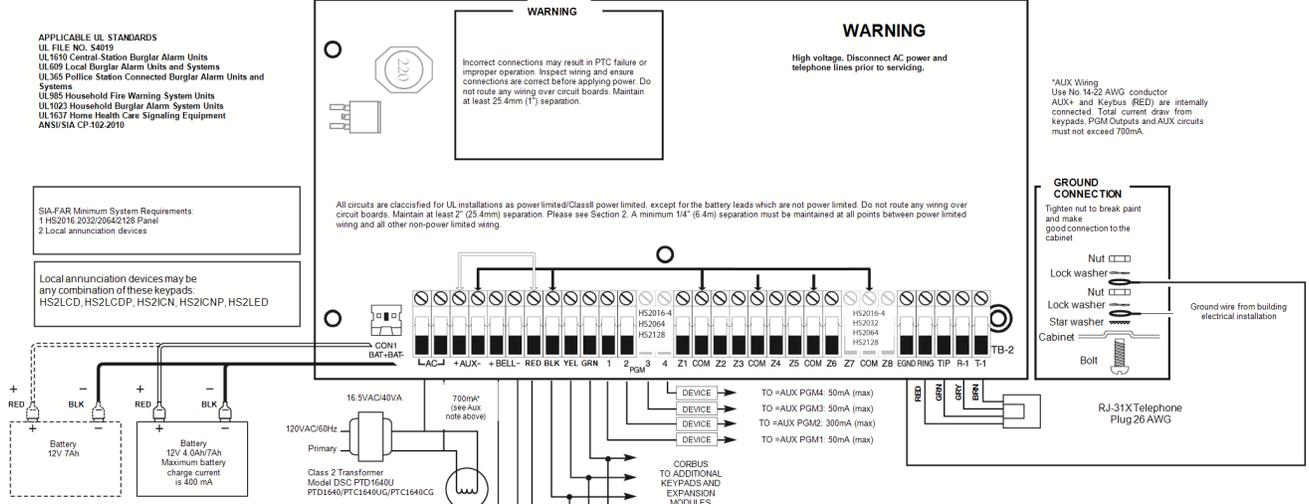
**NOTE:** Battery capacity for 4h standby is at least 4Ah. (Max. Aux current must not exceed 700mA).
