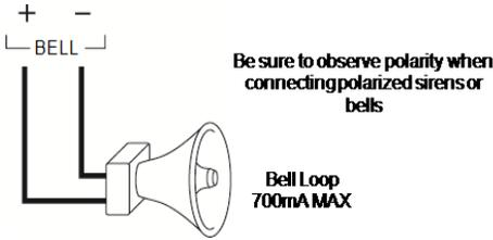
**Figure 2-13 Bell Wiring**
