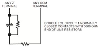
**Figure 2-11 DEOL Wiring**
