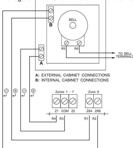
wiring is correct, and also check the Keypad/Auxiliary Supply fuse. If the fuse is open, check for a short between the Keypad's red and black leads before replacing the fuse.
