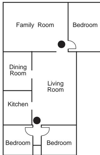
**Figure 4:** Smoke detector mounting and “dead” air space. The smoke from a fire generally rises to the ceiling, spreads out across the ceiling surface and begins to bank down from the
