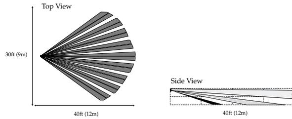
For optimum detection, the BV-300P should be located so that the expected path of intrusion is between 10ft - 40ft (3m-12m) in front of the detector.
