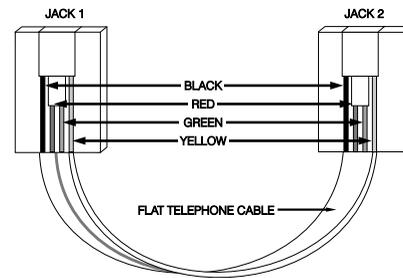
**NOTE:** Do not use a 'Swapped', 'Flipped' or 'Crossover' cable as it will not work with the ESCORT4580. To verify whether you have the correct type of cable, plug in the PSC04 (PL513). The red LED should turn ON. Connect the telephone cable to both the PSC04 (PL513) and the ESCORT4580. If the LED on the PSC04 (PL513) turns OFF and remains unlit, you are using the wrong type of cable.
