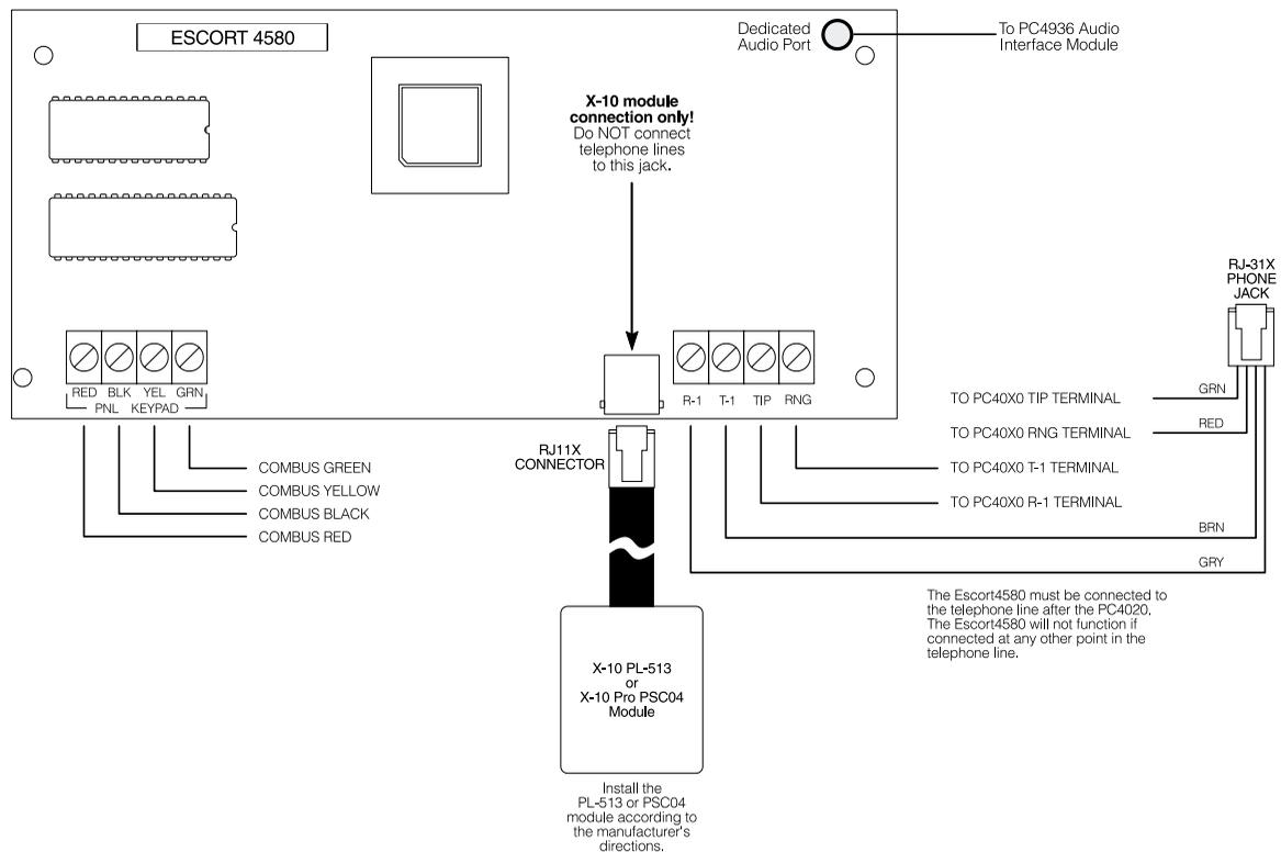
**NOTE:** If there is a PC4936 on the system, connect the modules to the telephone line as shown below.
