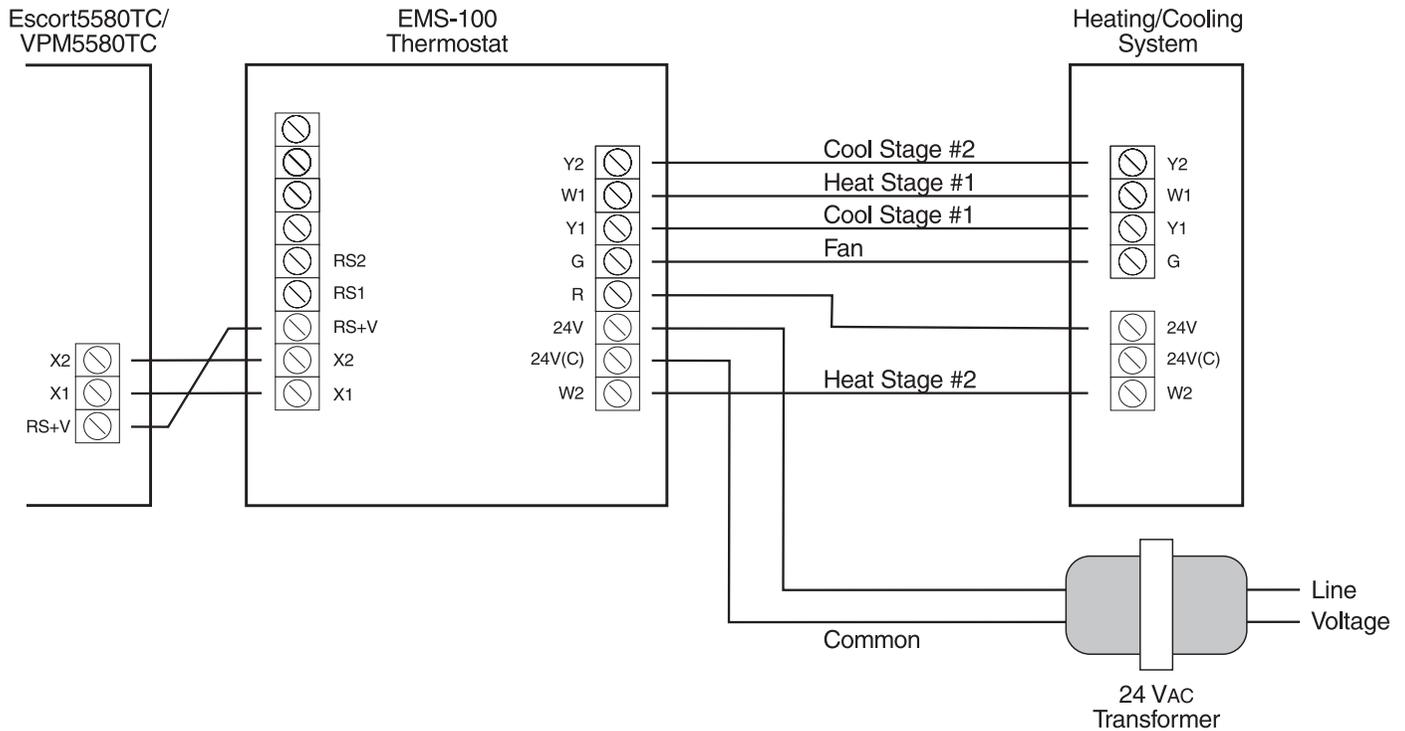
**⚠ Remove the internal jumper on the EMS-100 between R and 24V before connecting the standalone transformer.**
