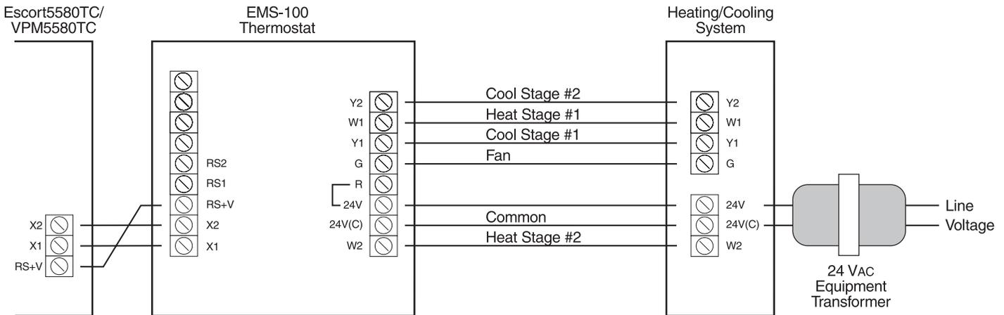
**⚠ Do not remove the jumper between R and 24V.**
