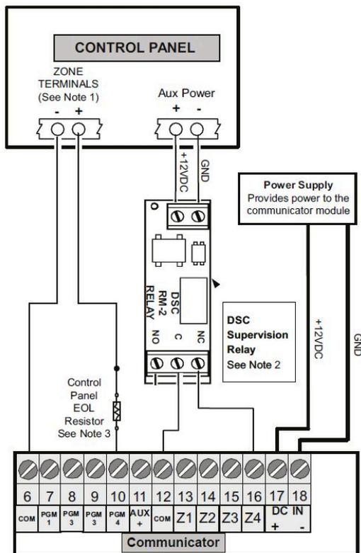
Program the zone/point as "Supervisory" type with keypad only annunciation when in alarm. Do NOT use a zone/point that is normally used for 2-wire smoke detectors. The power supervision relay (RM-2 or RM1C) is only used when the 3G4010CF/LE4010CF is not powered by the control panel. When the radio is powered by the control panel, the relay is not required since a loss of input power will generate a signal to the CMC. Output 4 on the 3G4010CF/LE4010CF must be set as "Active High" (default).
