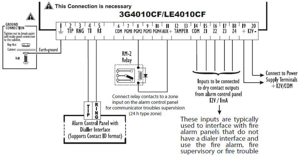
**Figure 4: Power Supply Wiring Diagram**
