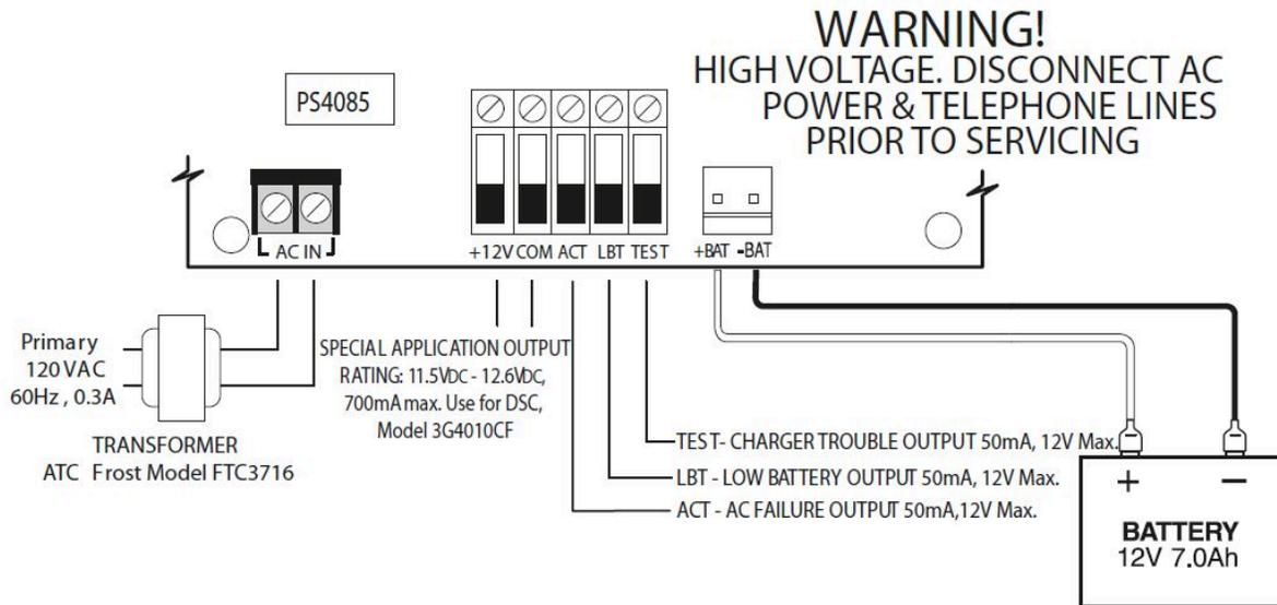
These outputs shall be connected to zone inputs of an alarm control panel in order to provide the required trouble supervision (visual and audible indication required at the control panel). The outputs are active low (switched to ground) and can be connected to a control panel directly or by using a listed supervision relay (suggested model: DSC, RM-2 or RM1C).
