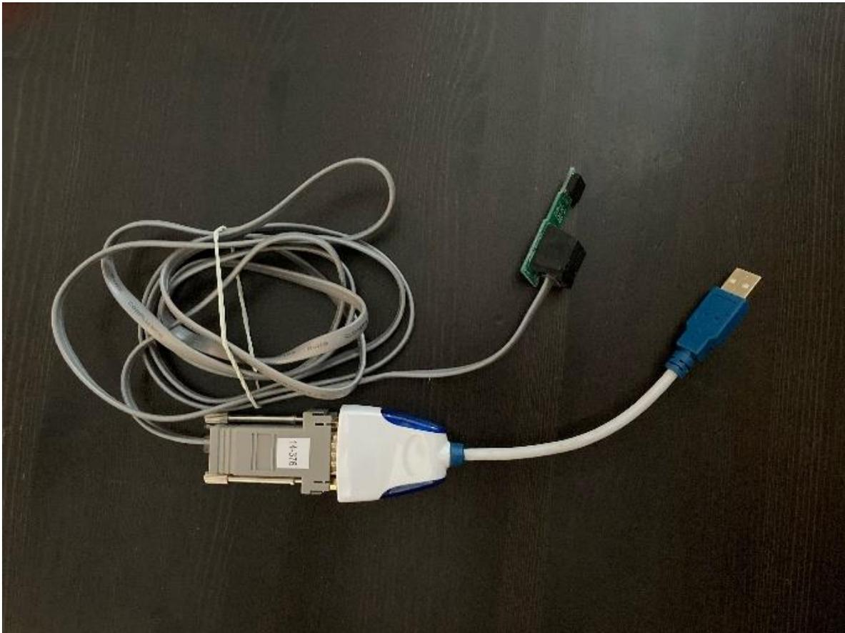
7. Pictured above is the kit called "PC-LINK-USB". This kit includes the PC-LINK header, cable, DB9 connector and USB to serial adapter. The USB to Serial adapter included in the PC-LINK kit is currently the only adapter recommended for use with the DLS 5 software.
