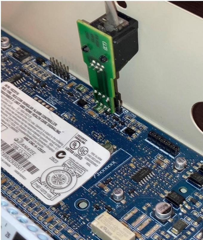
8. Notice the orientation of the 4 pin PC-LINK header on the NEO **PCLINK 2** five pin connector. Typically when downloading programming changes to the NEO control panel, you would connect to the PCLINK 1 pins. When doing a firmware update, you **MUST** connect to the **PCLINK 2** pins. The header must be connected on pins 1 to 4 from left to right. Pin 5 should be sticking out along the right side the PC-LINK header as in the photo.
