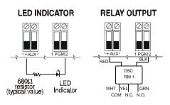
**IMPORTANT:** Minimum 6.4mm (1/4") separation must be maintained between RM-1 circuits and all other wiring
