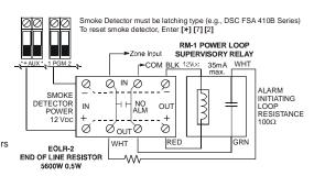
Compatible 4-wire Smoke Detector DSC FSA-410B Series
