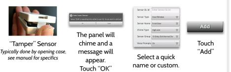
**NOTE**: Image Sensors are placed in "pairing mode" by removing and replacing the batteries. See installation manual for details.
