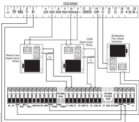
NOTE: Use EOL resistor in parallel with N.C. contacts of the relay connected to PGM4
