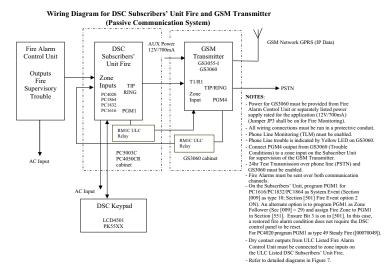
Figure 7 - DSC Subscribers' Unit Fire and GSM Transmitter Mounted Remotely
