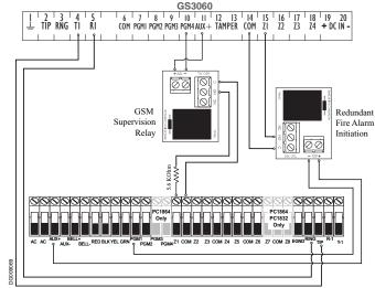
NOTE: Use EOL resistor in series with N.O. contacts of the relay connected to PGM4
