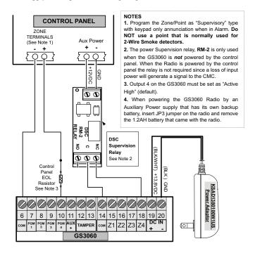
The following wiring diagrams (Figures 5 to 8) are examples of ULC Listed Fire Monitoring Installation connections.
