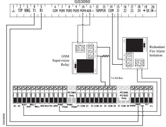
NOTE: Use EOL resistor in parallel with N.C. contacts of the relay connected to PGM4
