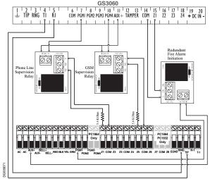
NOTE: Use EOL resistor in series with N.O. contacts of the relay connected to PGM4
