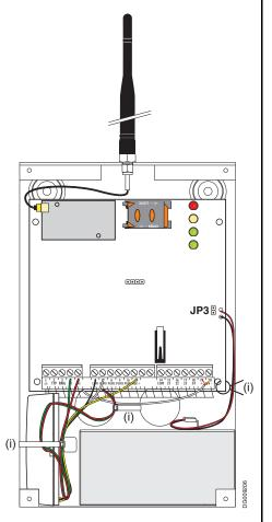
All circuits are classified for UL installations as Power Limited / Class 2 Power Limited except for the battery leads which are not power limited. Do not route any wiring over circuit boards. Maintain at least 1" (25.4mm) separation. A minimum 1/4" (6.4mm) of separation must be maintained at all points between Power Limited wiring and all other non-Power Limited wiring. Route wires as indicated above.
