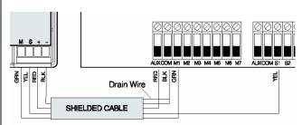
\* Connect drain wire to the COM terminal of PC5936 OR the black terminal of the station - NOT BOTH
