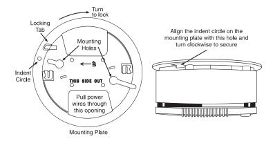
Locate the smoke alarm mounting plate on the wall or ceiling and mark all desired screw locations. Use the supplied wall anchors for all screw locations. When the anchors have been placed, secure the mounting plate to the ceiling or wall.
