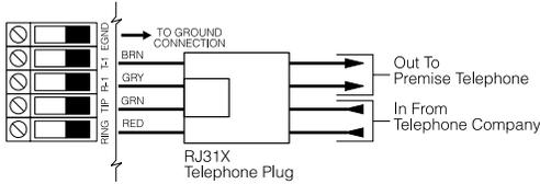
Connect the PC5020 and modules that use the telephone line(s) in the following order:
