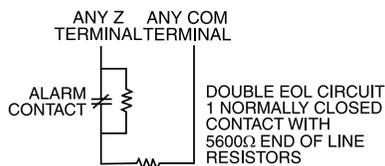
**NOTE:** If the Double EOL supervision option is enabled, all hard-wired zones must be wired for Double EOL resistors, except for Fire and 24 Hour Supervisory zones.
