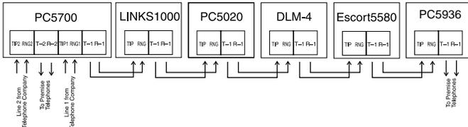
For example, if you are installing a PC5020 with a LINKS1000/ GSM1000 and a PC5936 Intercom module, connect the incoming line to the LINKS1000, then from the LINKS1000 to the PC5020, then from the PC5020 to the PC5936 Intercom and then from the PC5936 to the house telephones
