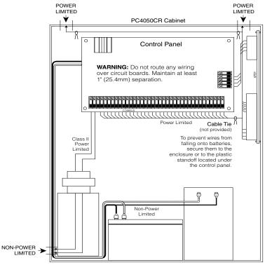
INSTALL BATTERY AND AC WIRING AS SHOWN ABOVE IMPORTANT: A minimum 1/4" (6.4mm) separation must be maintained at all points between battery/primary AC wiring and all other wiring connections.
